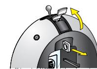
Lift the locking handle and remove the capsule holder.
