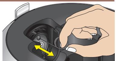
Unblock the injector with the cleaning needle.
