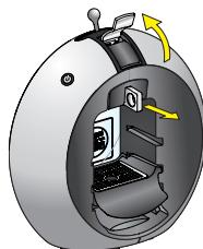
Then lift the locking handle and remove the capsule holder.
