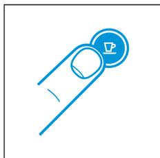
1. With machine being turned off, press and hold the Espresso button for 3 seconds.
