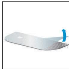
1. Remove the plastic film from the drip grid.
