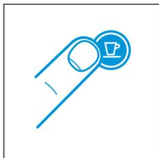
1. With machine being turned off, press and hold down the Lungo button for 5 seconds.
