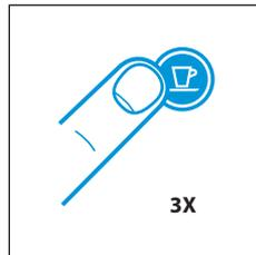
6. Press the Lungo button to rinse the machine. Repeat 3 times.
